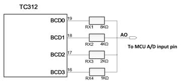
When using the BCD port to generate analog voltage, the corresponding relationship between the key and the AO voltage is as follows:
